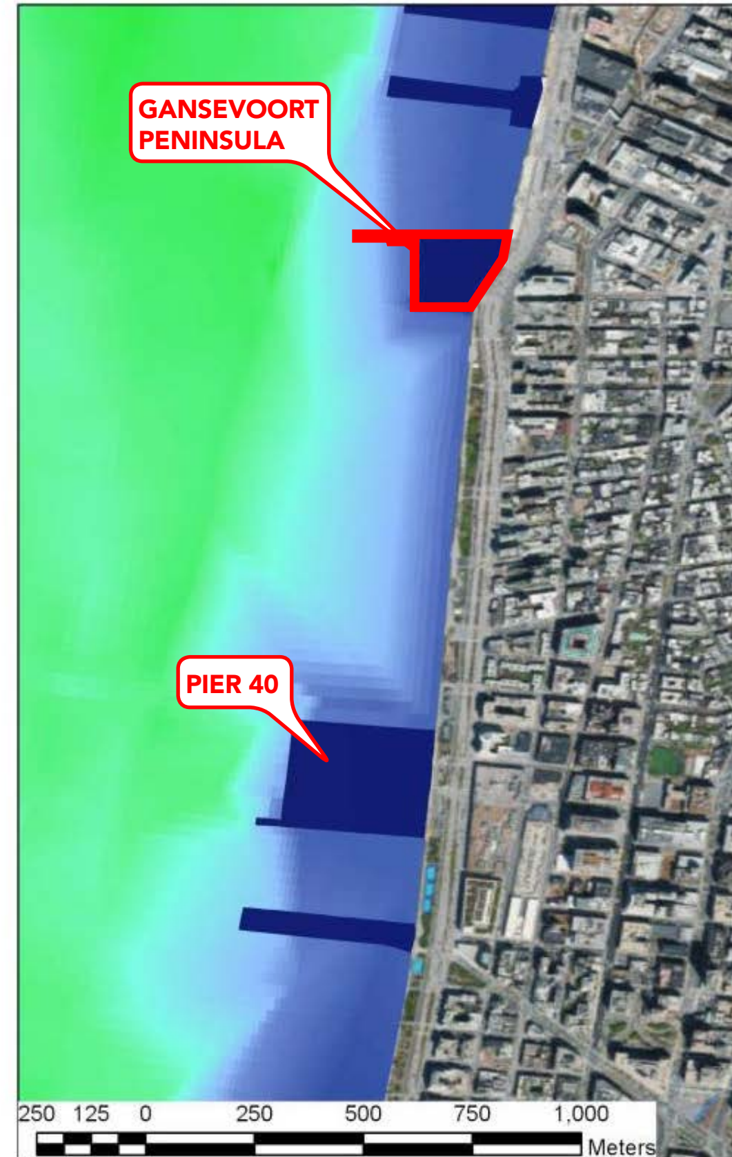
Delft3D bathymetry model used for wave modeling
