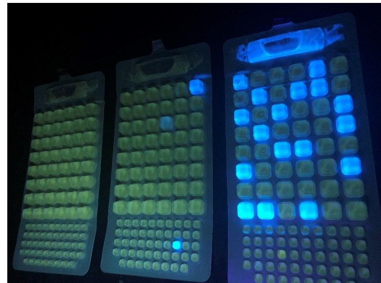
Fig. 2 (below) | Three Enterolert* Quanti-trays* with varying levels of Enterococcus contamination (blue fluorescence)
