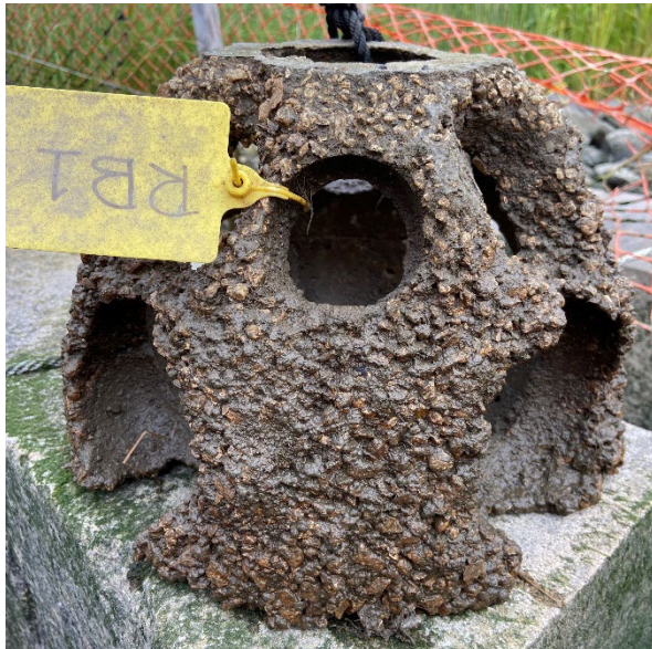
Fig. 8 | A miniature reef ball that is seeded with oyster spat, ready for deployment in the salt marsh.
