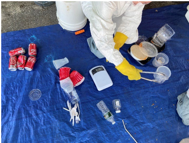
Fig. 3 | Plastics are sorted by resin identification codes (RIC) as they are weighed.
