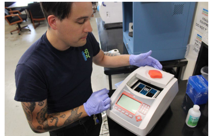
Fig. 6 | River Project staff loading thermocycler with DNA extractions for PCR.
