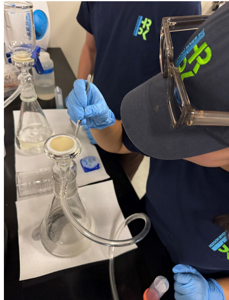
Fig. 5 | River Project staff performing vacuum filtration of May 2025 Pier 40 & Governor’s Island water samples.
