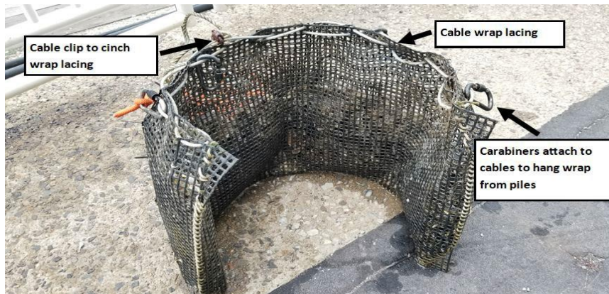
Fig. 2 | A standard oyster wrap with key components labeled.
