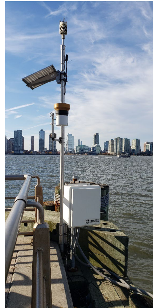
Fig. 1 | Pier 25 HRECOS station with Vaisala WXT series weather sensor, solar panel, and telemetry equipment enclosure visible.
