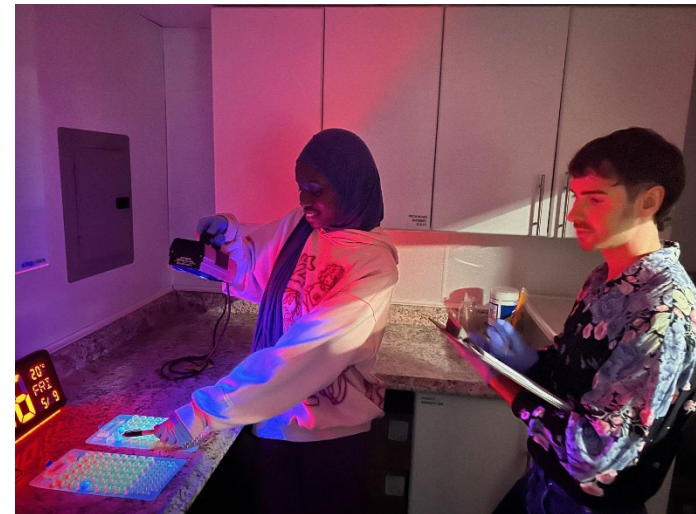
Fig. 4 | HRPK staff and CUNY interns analyzing the results of a Quanti-tray water sample after incubation.
