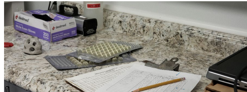
Fig. 6 | IDEXX Quantitrays are enumerated using and MPN value chart are pictured along with a completed data sheet from testing. after 24-26 hrs of incubation at 41C.
